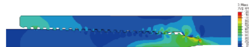
The low stress design of the joint makes TP-G4 the best choice for corrosive environment applications.
