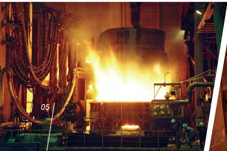
Electric Arc Furnace (EAF)
